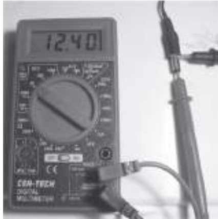
Checking the voltage of the plug
